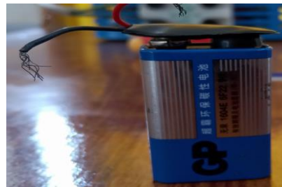
Fig. 9 9v Battery Source for Powering USB 2.0 Arduino Connecting Cable.
