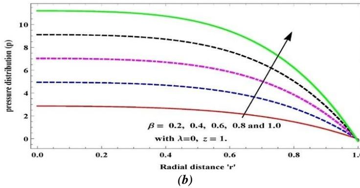
Figure 7: Impact of slightly viscoelastic parameter on pressure distribution with (a) slip condition (b) No-slip condition.
