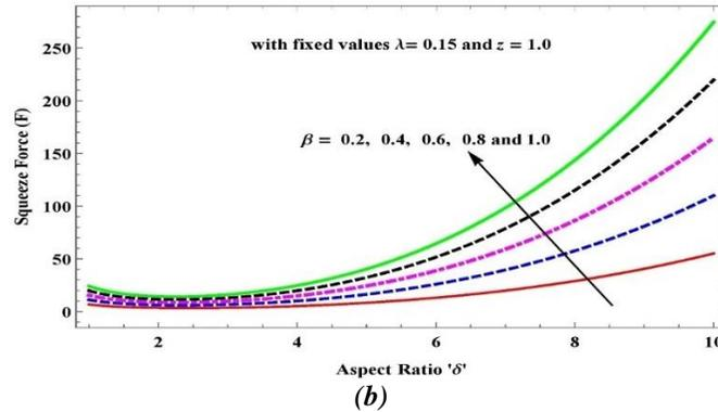
Figure 8: Impact of (a) slip parameter with  $\beta = 0.3$  (b) slightly viscoelastic parameter with  $\lambda = 0.15$  on squeeze force.
