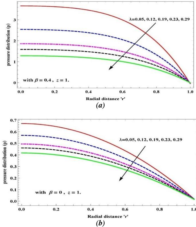
Figure 6: Impact of slip parameter on pressure distribution of (a) Slightly viscoelastic fluid (b) Viscous fluid.
