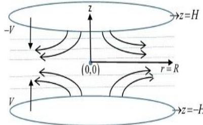
Figure 1: Squeeze flow between two Circular disks (Muravleva, 2018)
