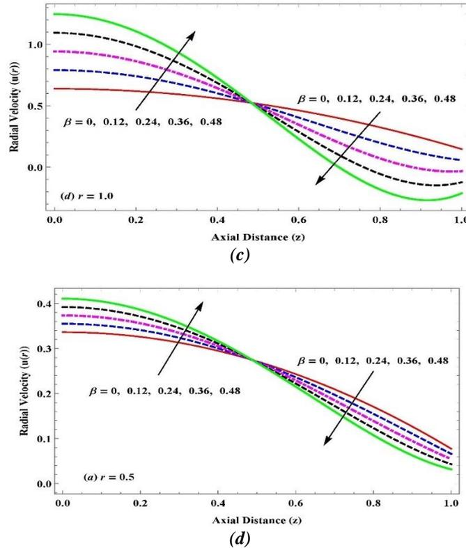
**Figure 2: Impact of slightly viscoelastic parameter ( $\beta$ ) on Radial velocity with fixed values of  $\delta = 0.1$ ,  $\lambda = 0.15$  at the following different radial points (a)  $r = 0.2$ ; (b)  $r = 0.5$ ; (c)  $r = 0.75$ ; (d)  $r = 1.0$ .**
