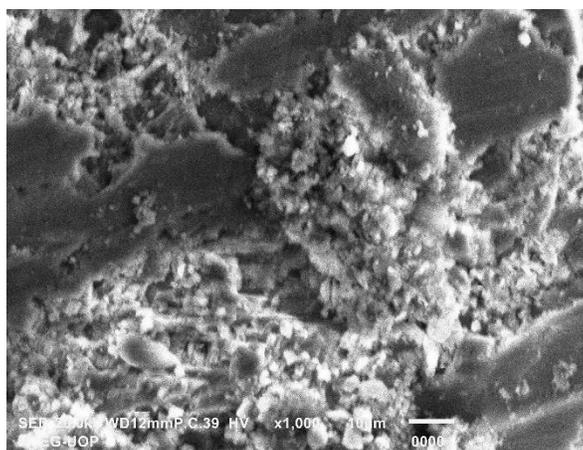
**Figure 16: SEM Image of Malakand Aggregates.**
