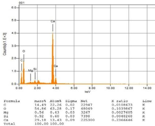
***Figure 21: Elements of Besai Aggregate.***
