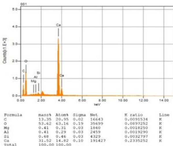
**Figure 19: Elemental Composition of Kohat Aggregate.**
