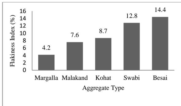
**Figure 6: Variation in flakiness index of aggregate.**
