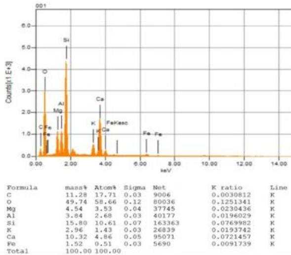
**Figure 17: Elemental Composition of Swabi Aggregate.**
