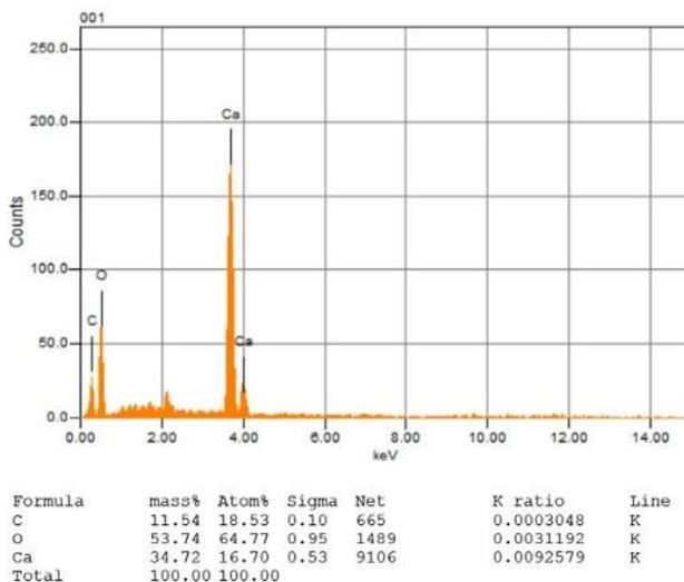
**Figure 15: Elemental Composition of Malakand Aggregate.**
