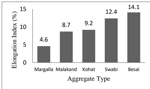
**Figure 7: Variation in elongation index of aggregate.**
