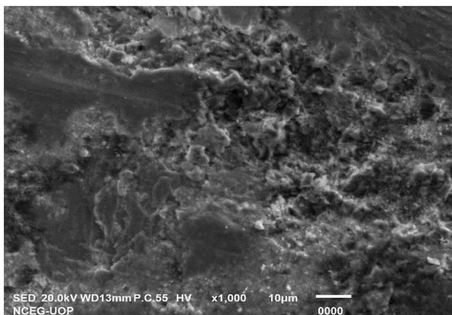
**Figure 14: SEM Image of Margalla Aggregate.**
