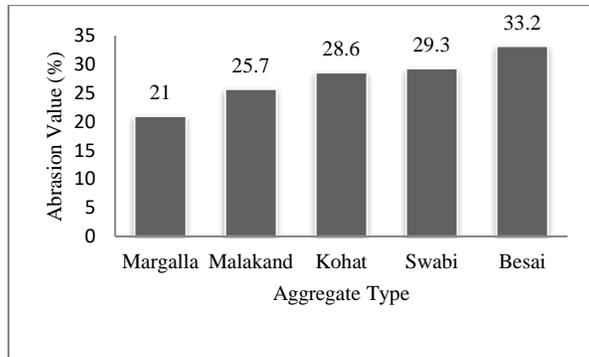
**Figure 5: Variation in abrasion values of aggregate.**
