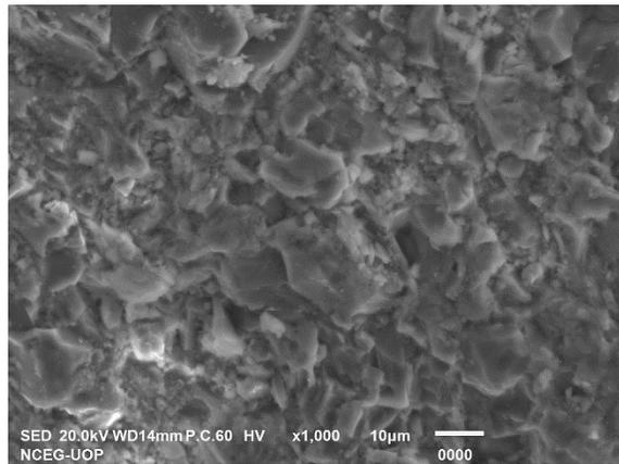
**Figure 18: SEM Image of Swabi Aggregate.**
