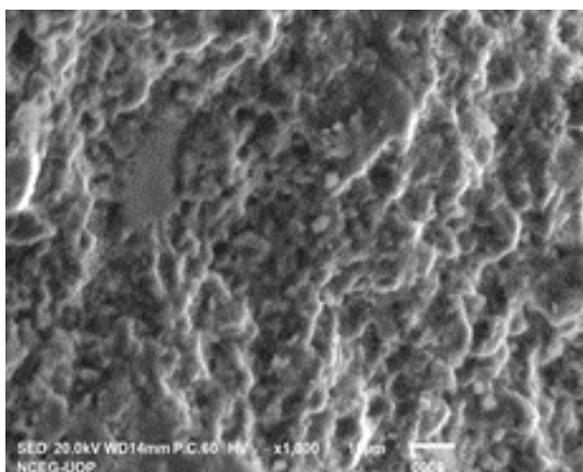
**Figure 20: SEM Image of Kohat Aggregate.**
