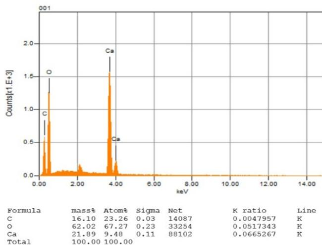
**Figure 13: Elemental Composition of Margalla Aggregate.**
