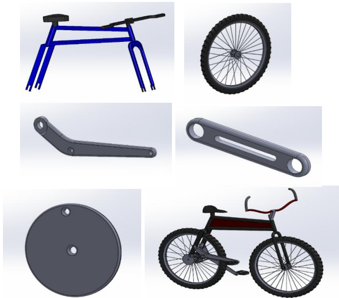
Figure 1: CAD model of frame, tyre, crank lever, drive lever, drive wheel and chainless bicycle.
