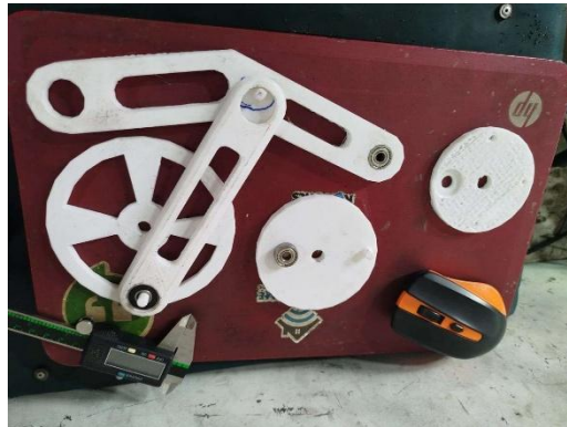
Figure 6: 3D printed parts of the Chainless bicycle.
