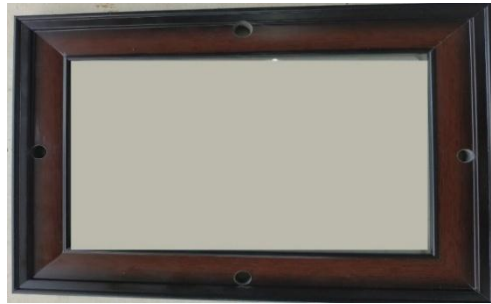
Figure 2: Integration Frame used to hold the Fresnel lens.
