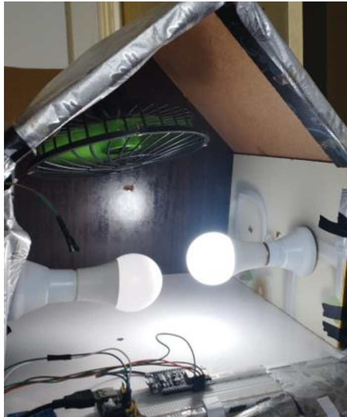
Figure 10: Hardware model for home appliances control via muscle sensor.
