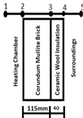
Figure 8: Plane wall with insulation.
